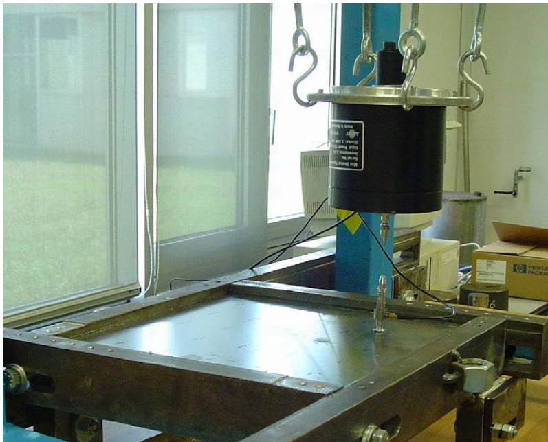
Fig. 2. Photograph of the experimental plate, connected to the shaker by the stinger and the load cell.
